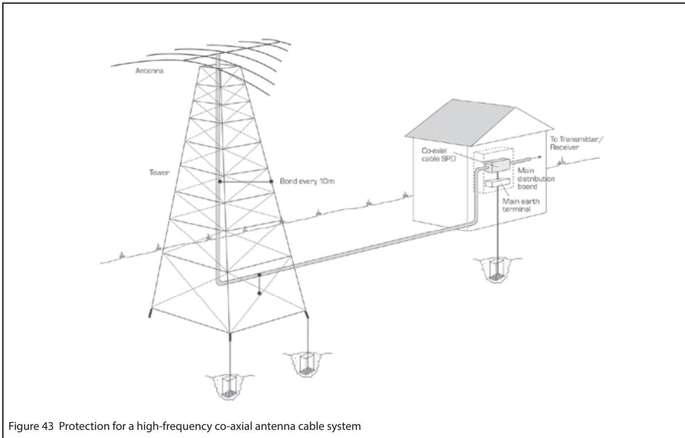
Figure 43 Protection for a high-frequency co-axial antenna cable system
