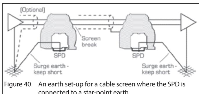
Figure 40 An earth set-up for a cable screen where the SPD is connected to a star-point earth
