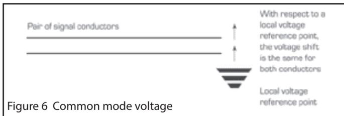
Figure 6 Common mode voltage
