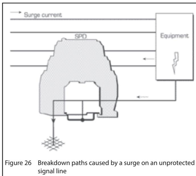
Figure 26 Breakdown paths caused by a surge on an unprotected signal line
