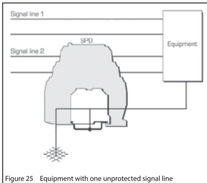
Figure 25 Equipment with one unprotected signal line
