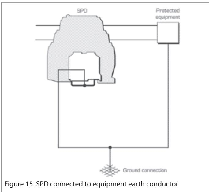
Figure 15 SPD connected to equipment earth conductor
