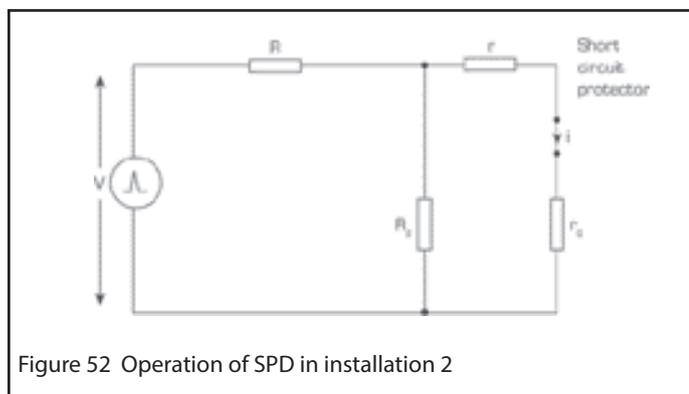
Figure 52 Operation of SPD in installation 2
