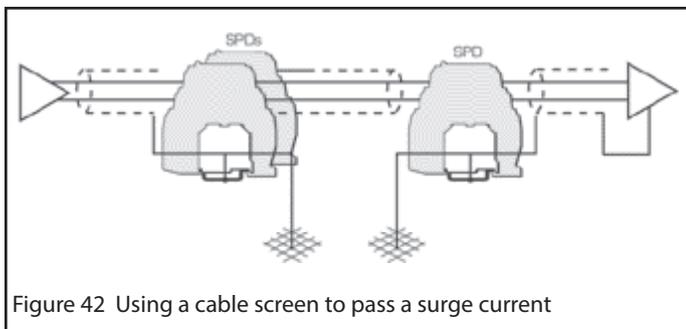
Figure 42 Using a cable screen to pass a surge current
