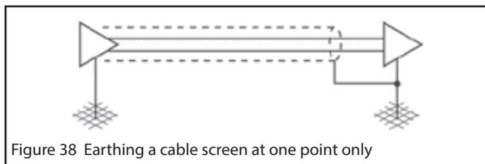
Figure 38 Earthing a cable screen at one point only
