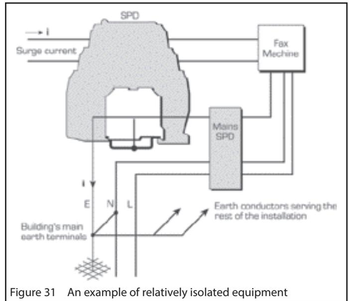
Figure 31 An example of relatively isolated equipment
