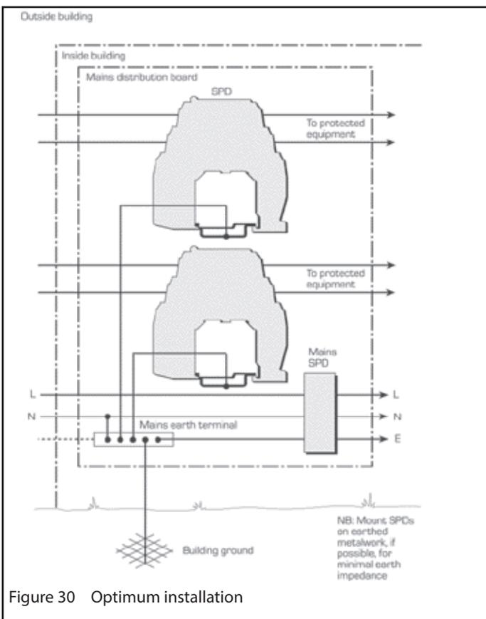
Figure 30 Optimum installation
