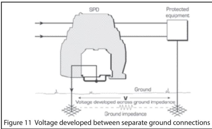
Figure 11 Voltage developed between separate ground connections
