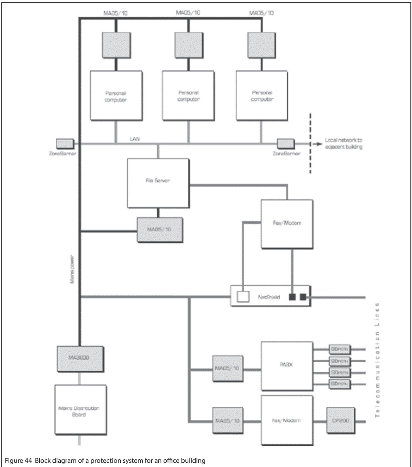
Figure 44 Block diagram of a protection system for an office building
