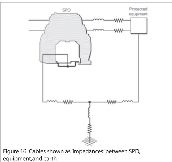
Figure 16 Cables shown as 'impedances' between SPD, equipment, and earth
