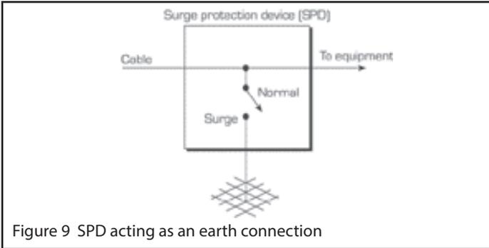
Figure 9 SPD acting as an earth connection
