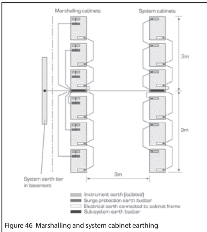
Figure 46 Marshalling and system cabinet earthing
