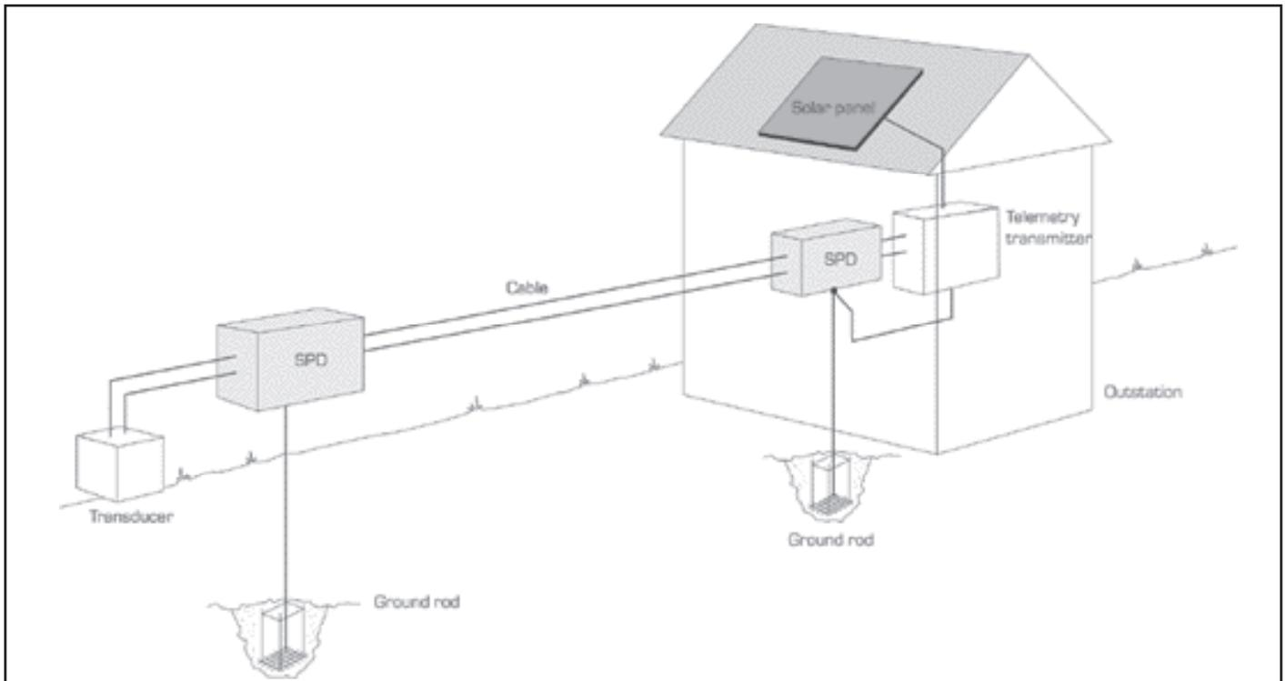
Figure 34 Outstation installation – with ground rod
