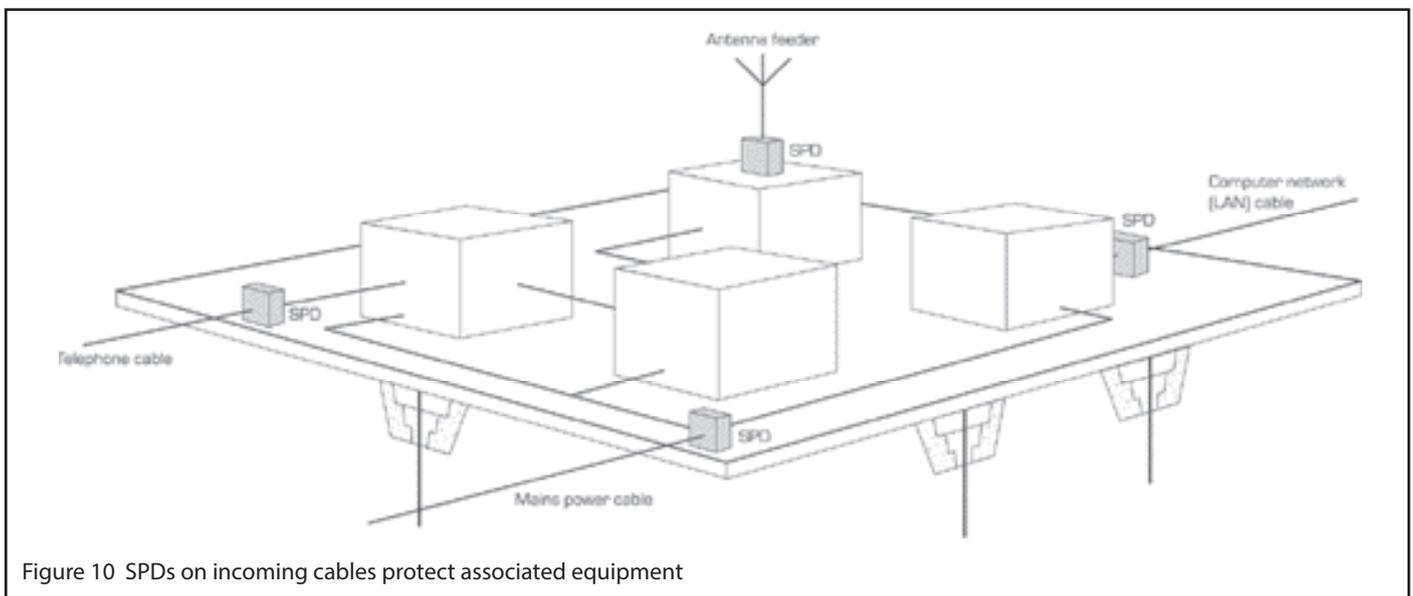
Figure 10 SPDs on incoming cables protect associated equipment
