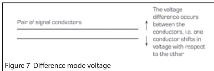
Figure 7 Difference mode voltage
