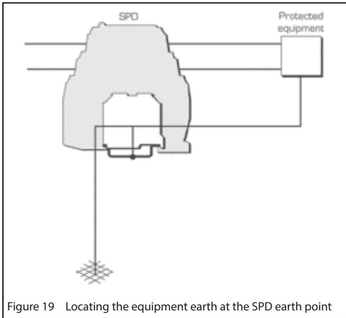
Figure 19 Locating the equipment earth at the SPD earth point
