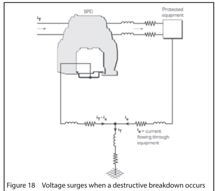
Figure 18 Voltage surges when a destructive breakdown occurs
