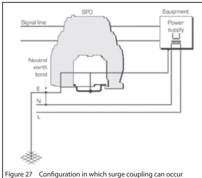
Figure 27 Configuration in which surge coupling can occur
