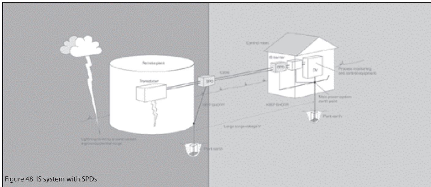
Figure 48 IS system with SPDs
