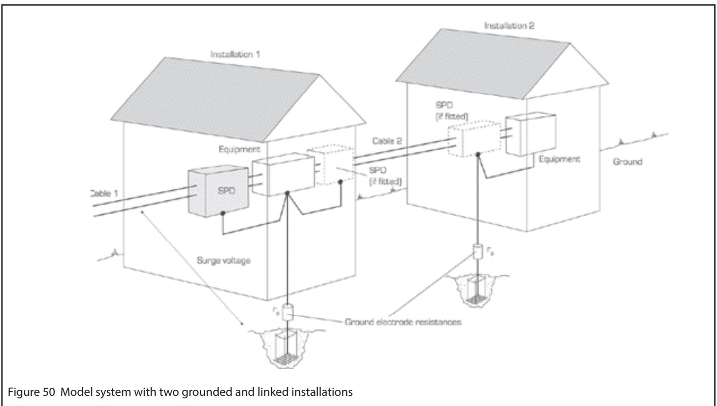
Figure 50 Model system with two grounded and linked installations
