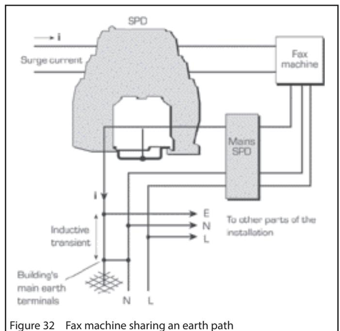
Figure 32 Fax machine sharing an earth path
