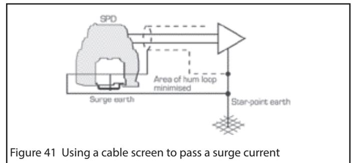
Figure 41 Using a cable screen to pass a surge current
