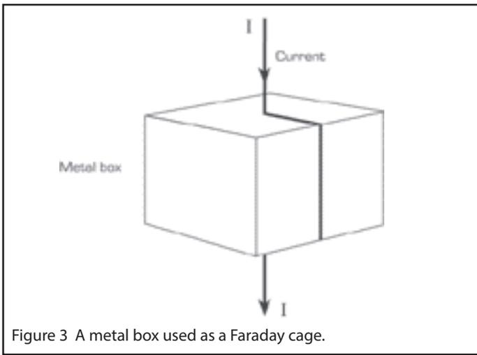
Figure 3 A metal box used as a Faraday cage.
