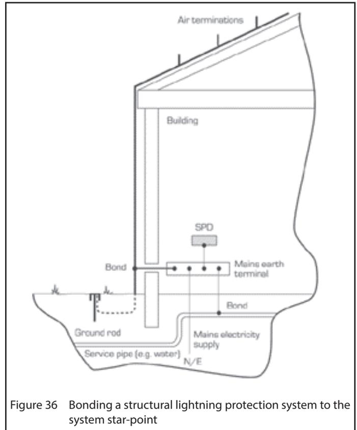
Figure 36 Bonding a structural lightning protection system to the system star-point
