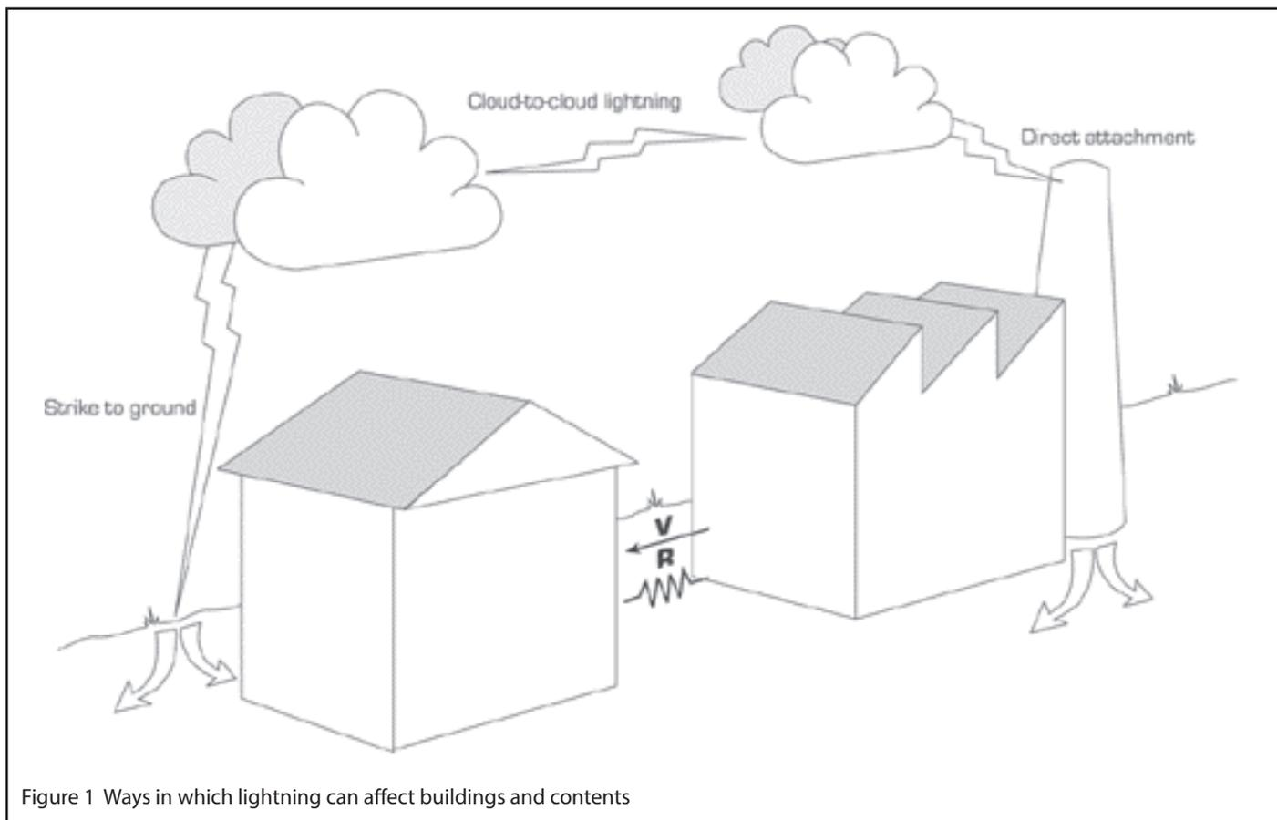
Figure 1 Ways in which lightning can affect buildings and contents
