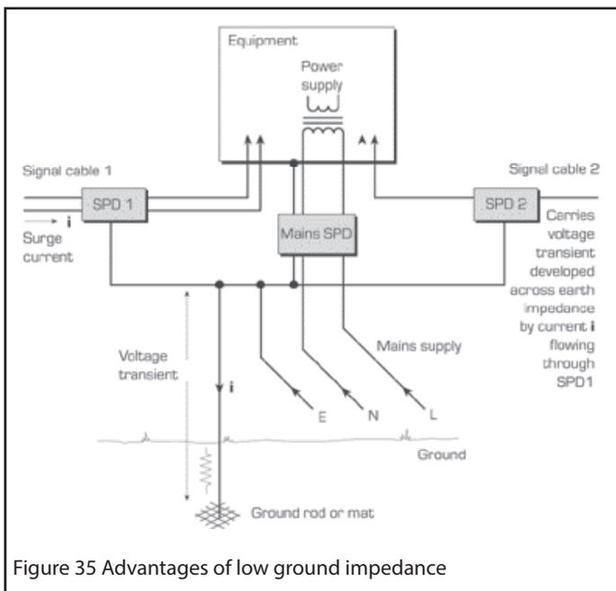
Figure 35 Advantages of low ground impedance
