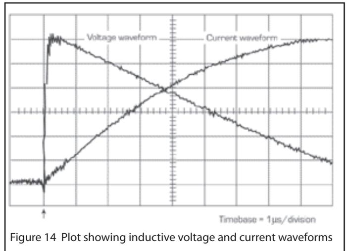
Figure 14 Plot showing inductive voltage and current waveforms
