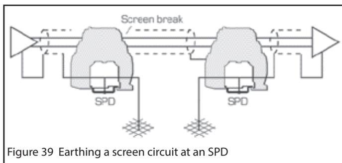
Figure 39 Earthing a screen circuit at an SPD
