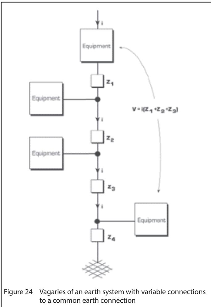
Figure 24 Vagaries of an earth system with variable connections to a common earth connection
