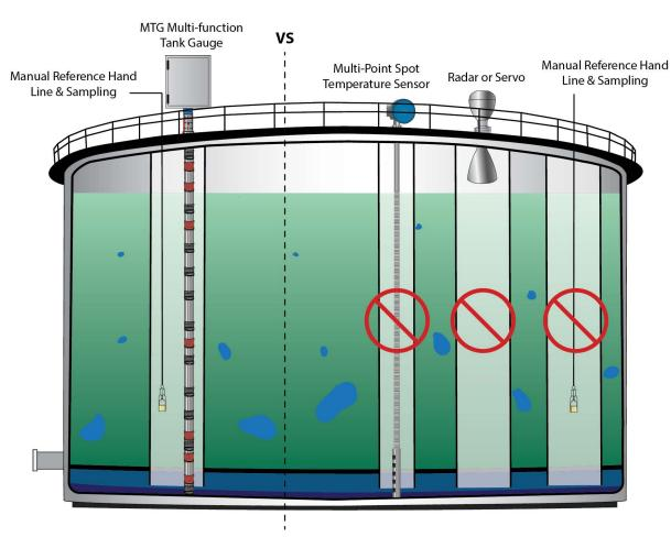
One tank entry (with or without gaugewell) providing entry for an ATG and manual reference hand lines & sampling at the same time. Thus, providing a point of direct comparison of the ATG and manual reference measurements (using the same physical location and product media) for calibration and checking the ATG accuracy.
