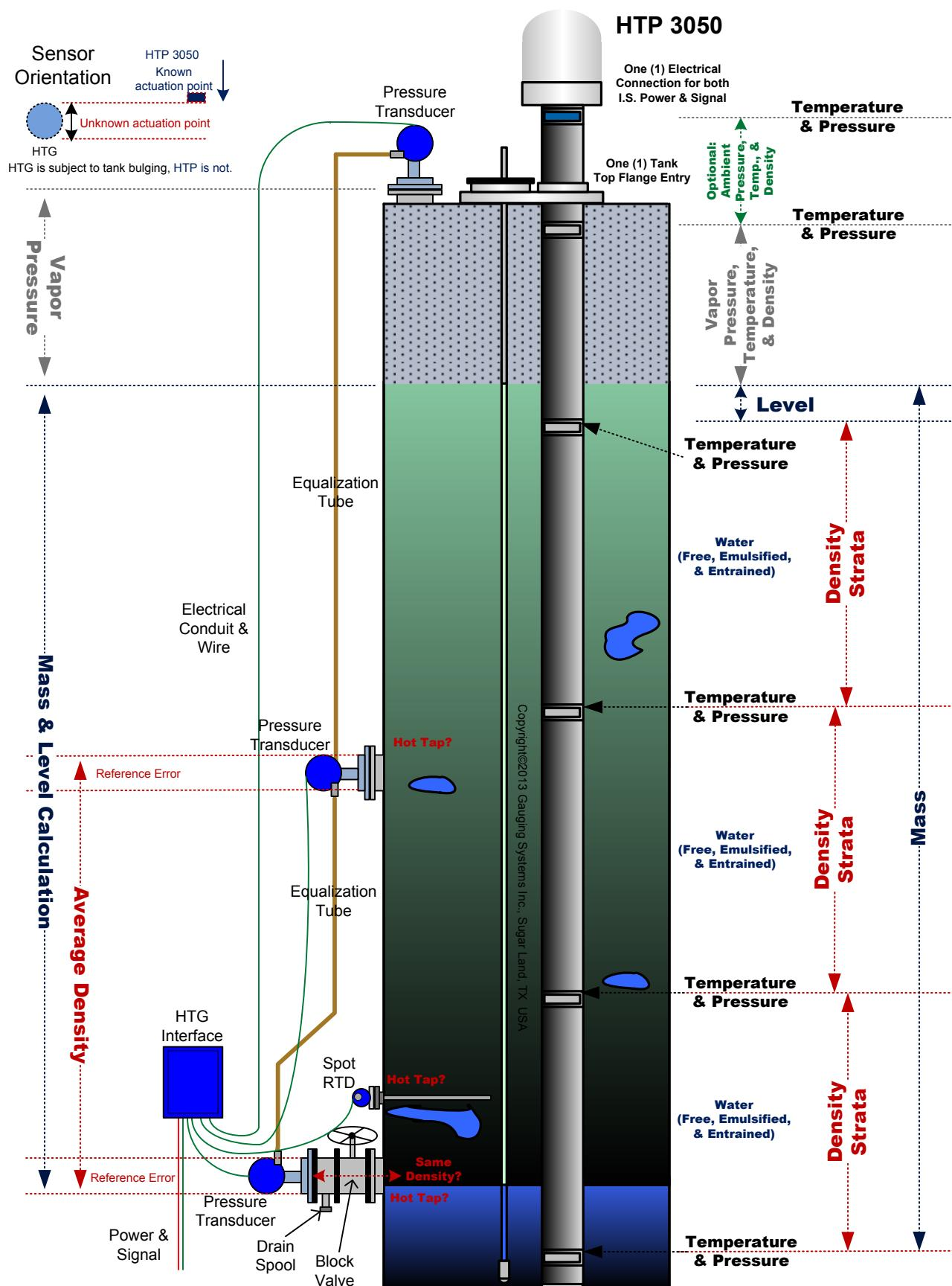
Volume by Hydrostatic Method - API MPMS Chapter 16.2
